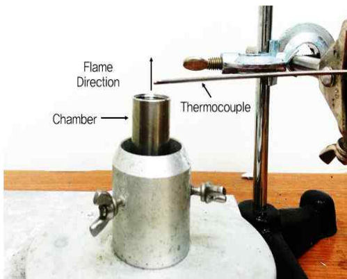
Fig. 3. Test setup for temperature measurements
