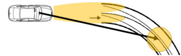
Fig. 11 Visibility Limit of Retroreflective Method
