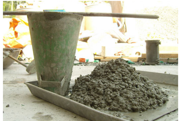
(a) Concrete Slump
