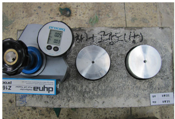
(c) Bond Strength Measurement by Pull-out Test
