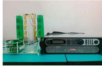
Fig. 6. Experimental environment for monitoring insulation resistances.
