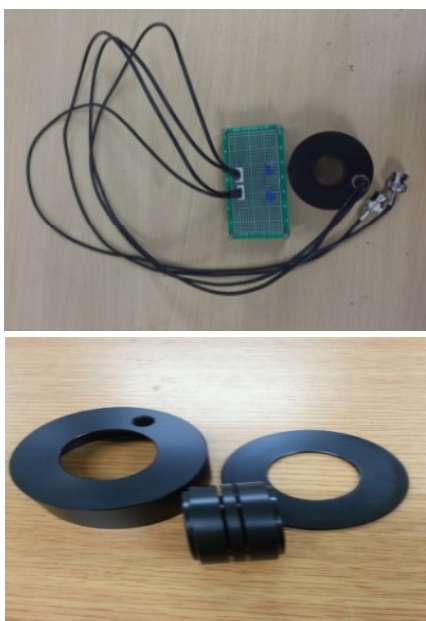
Fig. 10 Home-made ECT bobbin probes
