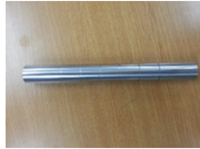
Fig. 2 Standard sample for detecting cracks
