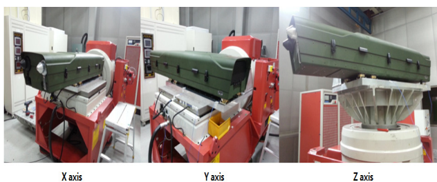
Fig. 13 Shock and vibration test setups for the launcher pod
