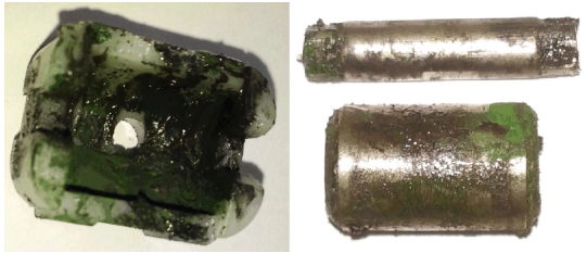
Fig. 6 Faulted lower roller of roller type door checker after the experiment
