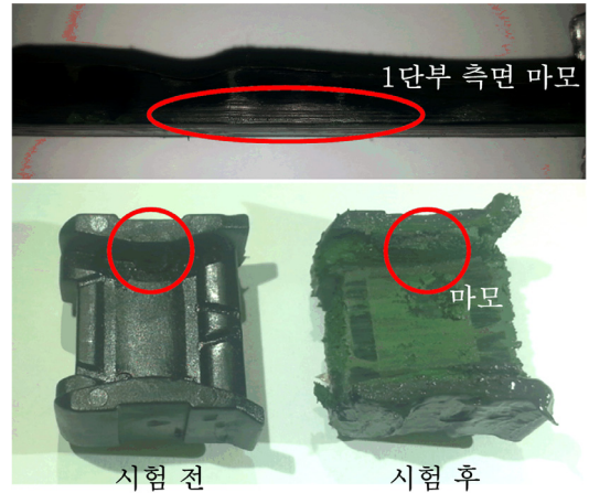
Fig. 7 Faulted lower slider in hybrid door checker after the experiment
