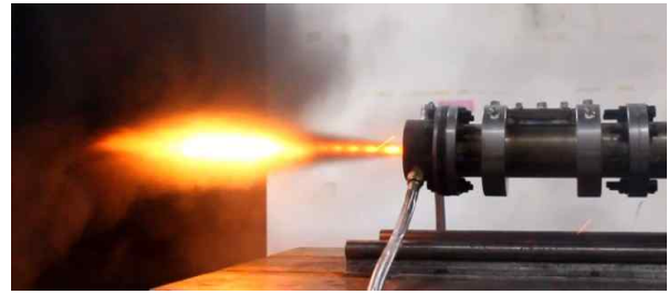
Fig. 7. Image of Secondary Combustion flame from Gas Generator
