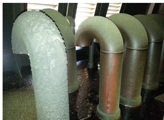
Fig. 2. The Goose-neck type of Air Vent Head.
