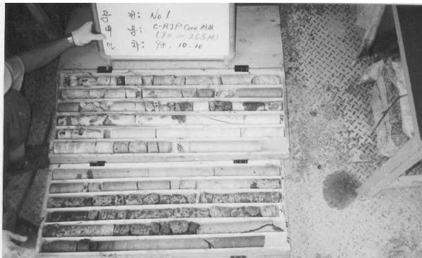
Fig. 9. Core sampling of the third test construction
