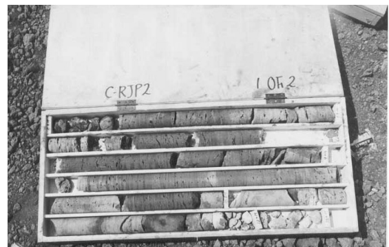
Fig. 8. Core sampling of the second test construction
