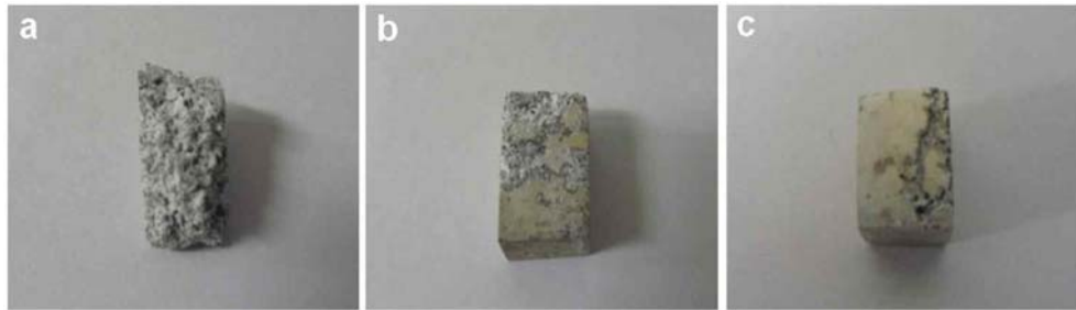
Fig. 7. Macroscopic images showing corroded surfaces of solution-treated (a) Mg-8%Al, (b) Mg-8%Al-0.5%Zn and (c) Mg-8%Al-1.0%Zn specimens after immersion in 1 M NaCl solution for 96 h.
