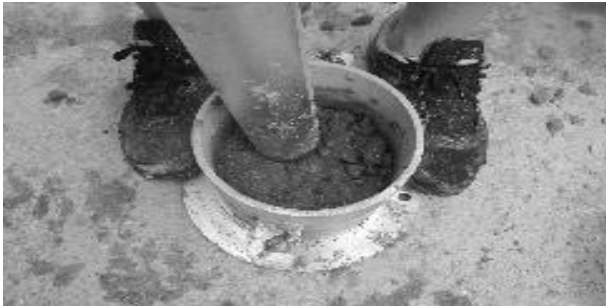
Fig. 4. Modified Proctor Test ASTM D1157
