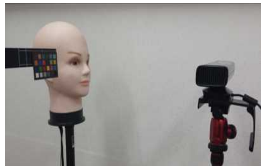
Fig. 1. Setup for 3D face measuring using Kinect sensors.
