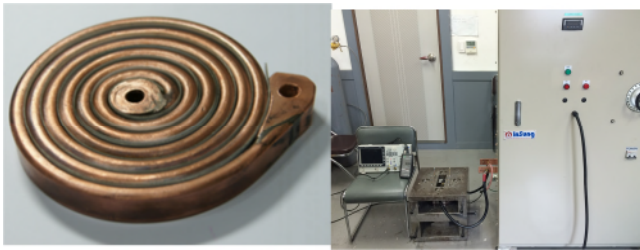
(a) Working coil (b) Actual equipment
