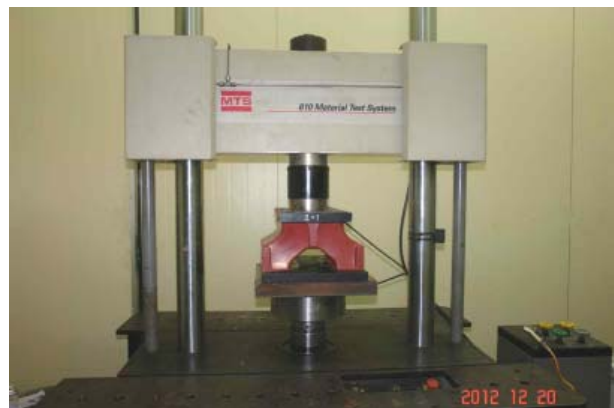
Fig. 1 Photo for deflection at upper rated load test
