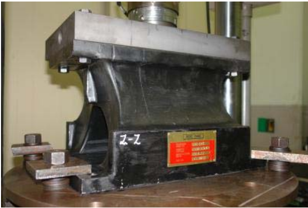
Fig. 12 Photo for static load deflection (tension)
