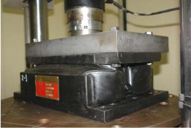
Fig. 13 Photo for static load deflection (compression)
