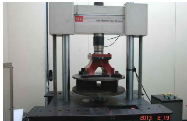
Fig. 5 Photo for static load deflection test
