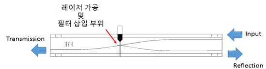
Fig. 6 Schematic diagram of optical waveguide.
