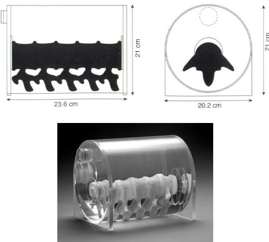
Figure 2 CT/X-RAY Phantoms 3D Spine Phantom Model 025(CIRS). This phantom included L-spine
