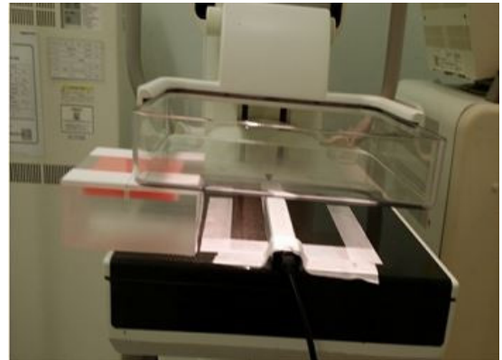
Figure 5 Radiolucency measurement by Unfors Xi dosimetry
