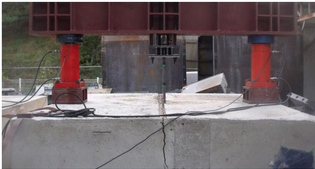
Fig. 8 Splitting failure of LA-3-100
