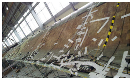
Fig. 4 Mounted sensors on the upper skin of blade
