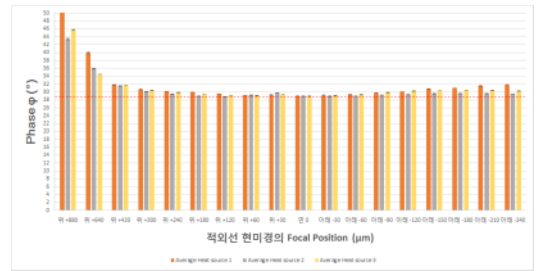
Fig. 11 Phase graph according to the focal plane position of an infrared microscope
