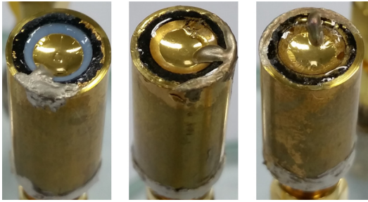
Fig. 1 Photo of the fabricated PVDF high frequency ultrasonic transducers for a PAM detector
