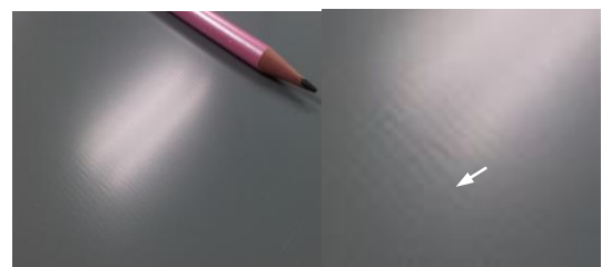
(c) Shape defects due to severe leveling
