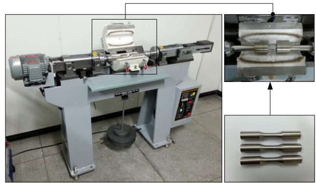
Fig. 7 Rotating bending fatigue machine testing machine for estimating S-N curve of STD11
