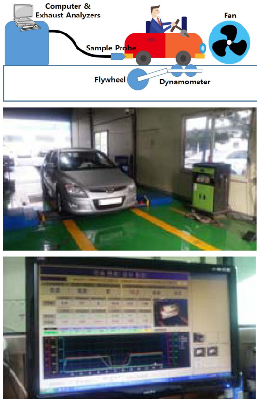
Fig. 1 Schematic diagram of experimental apparatus and test picture
