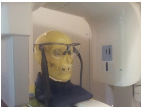
Figure 1(a) Experiment arrangement of the lead glasses & thyroid gland protective gear
