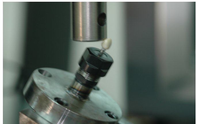
Fig. 4. Measurement of fracture strength. The load was applied 3mm below the incisal edge at an angle of 30°.
