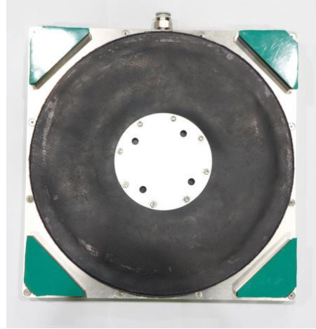
Fig. 9 Completed air cushion transporter.
