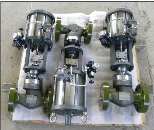
Fig. 1 Test air operated valve
