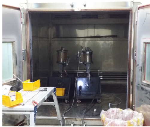
Fig. 6 Thermal aging chamber and test valve
