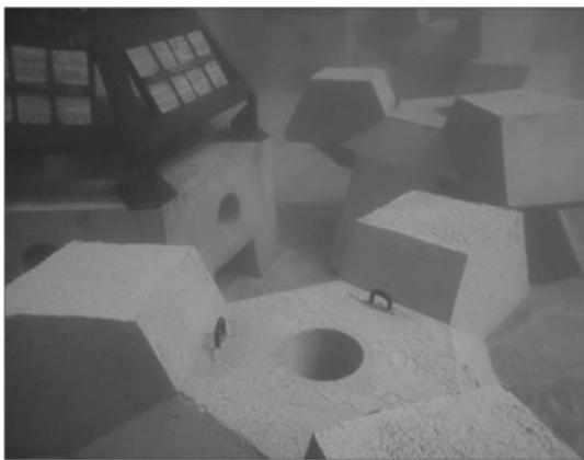
Fig. 7 Low Carbon Fish Shelters, 'Triton', made of Steel Slag
