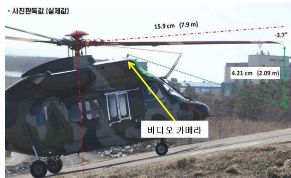
Fig. 12. Flapping angle in Nose-Up Slope Landing
