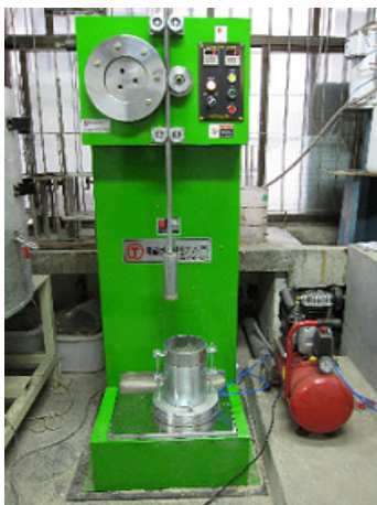
Fig. 3. Automatic compactor for standard B compaction test
