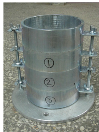
Fig. 4. Three separate layers of compaction mold
