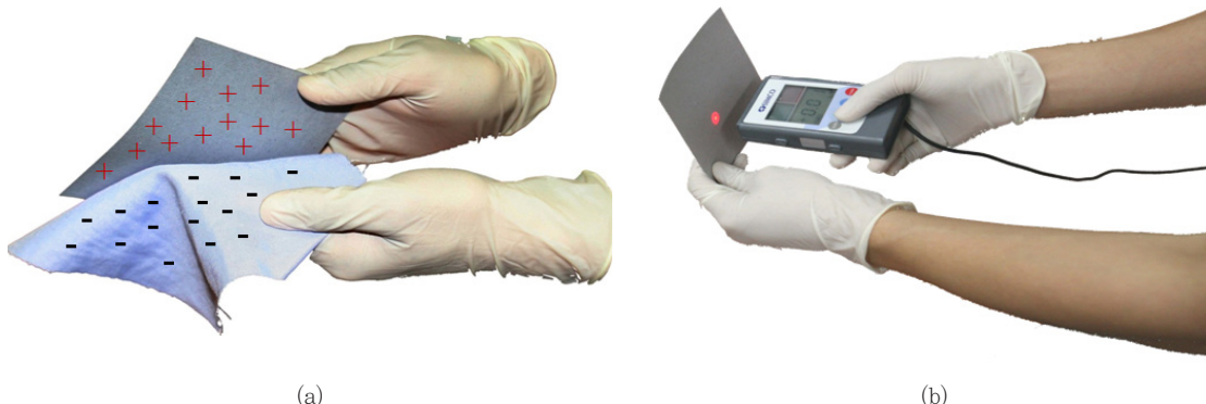
Fig. 2. Generation of static electricity (a) and measurement of charging voltage (b).
