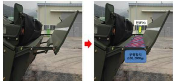
(c) Schematic of the stationary fin and buoyancy devices installation
