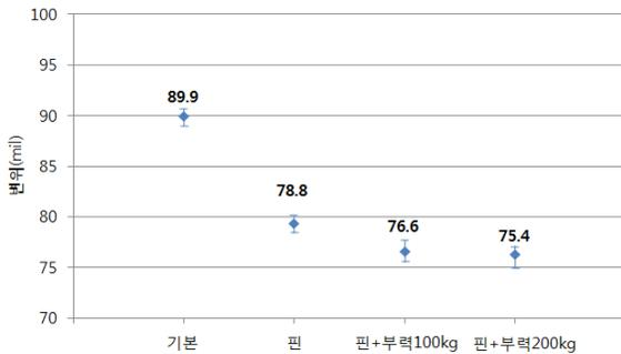
Fig. 6. Displacement variation during rapid reduction of speed at 'section III' in Fig. 5
