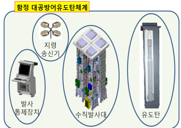
Fig. 1. Short-Range air defense missile system configuration
