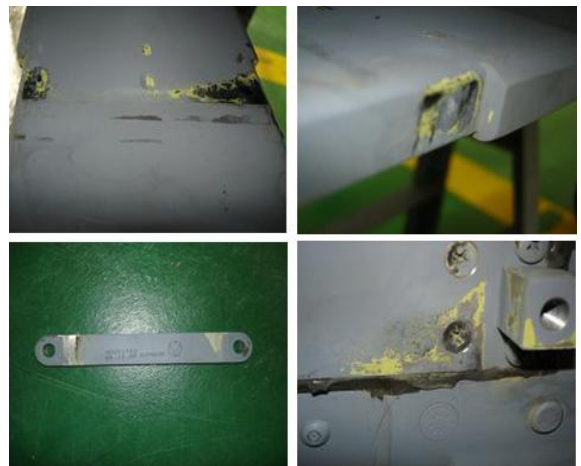
Fig. 6. Frictional wears on the strut components
