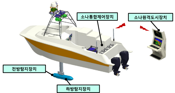
Fig. 5. Overview of sonar system
