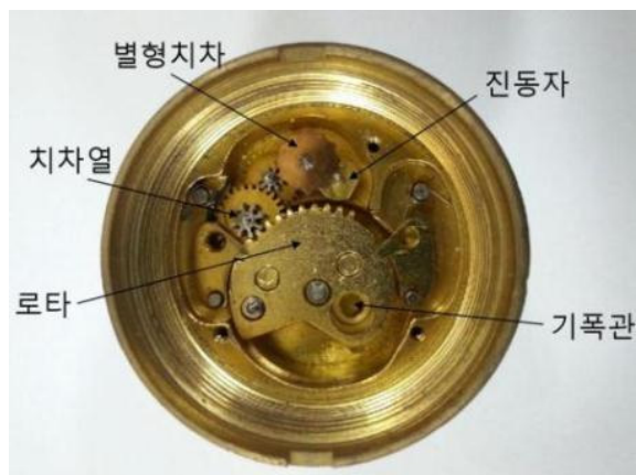
Fig. 3. Internal structure of safety & arming device
