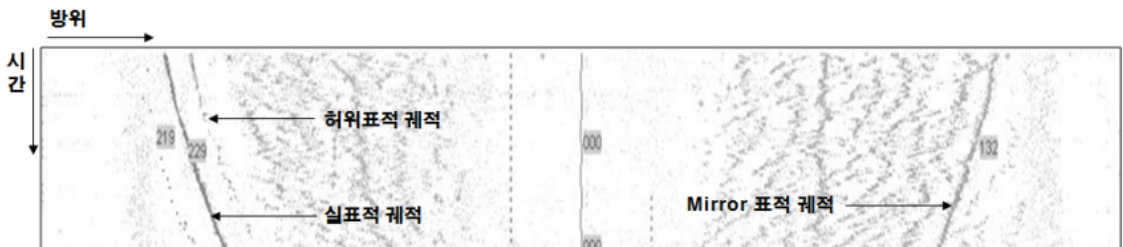
Fig. 2. Real target track and ghost target track displayed on waterfall
