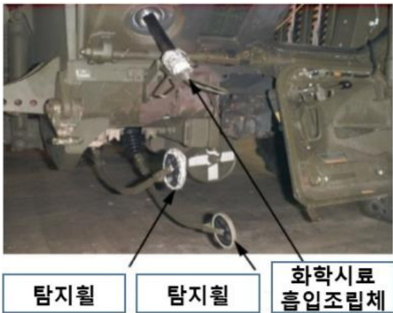
Fig. 1. Surface chemical detection using the DWSS of reconnaissance vehicles
