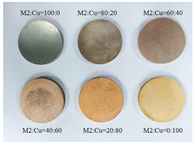
Fig. 1 Photos of FGM specimens
