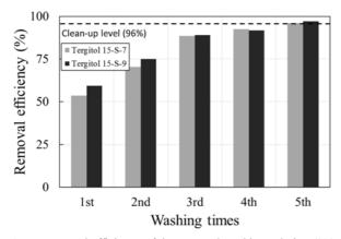
Fig. 5. Removal efficiency of the repeated washing solution (2% surfactant solution).
