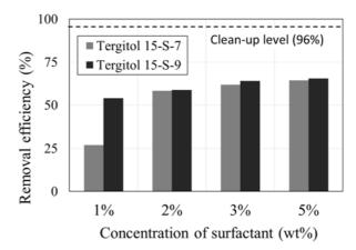
Fig. 4. Removal efficiency of the washing solution with different surfactant concentrations.
