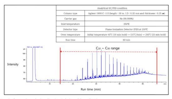
Fig. 1. GC peak of contaminants in the soil and analytical conditions of GC/FID.
