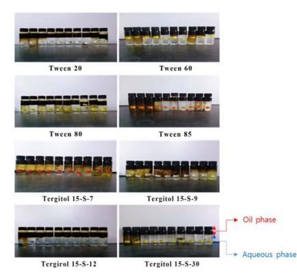
Fig. 2. Separated crude oil phase (top) and aqueous phase (bottom) of the mixed surfactant solution in a vial.
