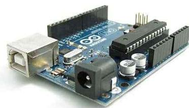
Fig. 1. Physical Computing Platform, Arduino
