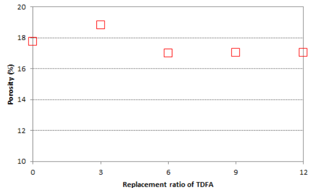
(b) Porosity with TDFA replacement
