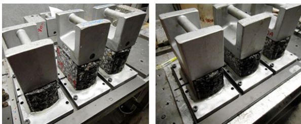
Fig. 6 Glued Samples with 4.5kg Curing Weights
