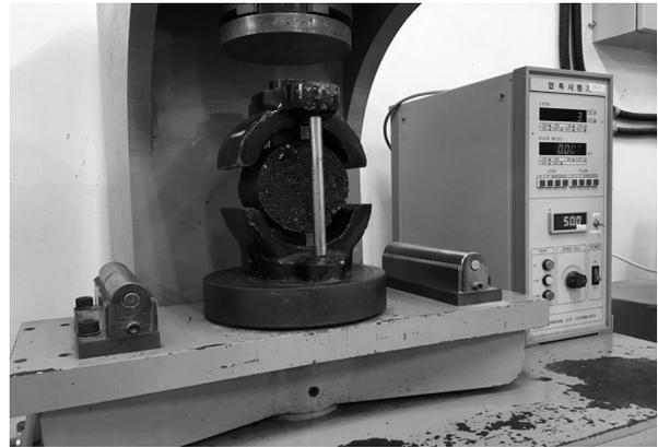
Fig. 6. Indirect Tensile Strength : ITS
