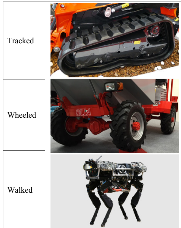
Fig. 1 Locomotion mechanism of robot lower body
