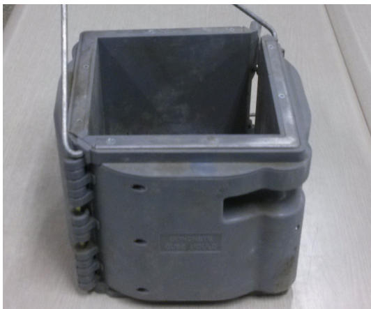
Fig. 2 Fabricating mold and test-piece (15×15×5 cm)
