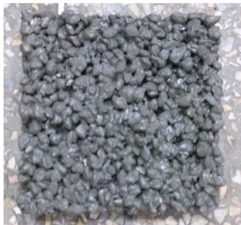
Fig. 2 Fabricating mold and test-piece (15×15×5 cm)
