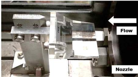
Fig. 5. Double compression ramp model
