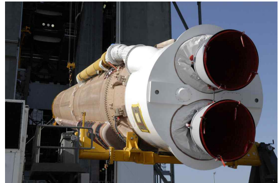
Fig. 2. RD-180 engine and Atlas V[6]
