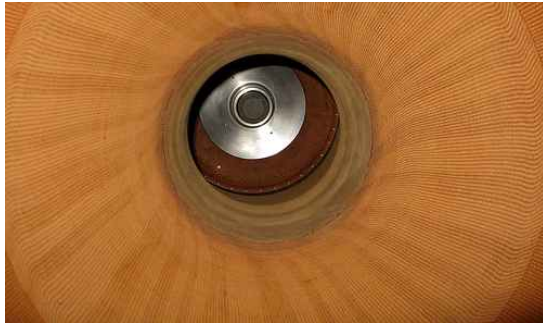
Fig. 5. LMDE, Lunar Module Descent Engine's pintle injector[10]
