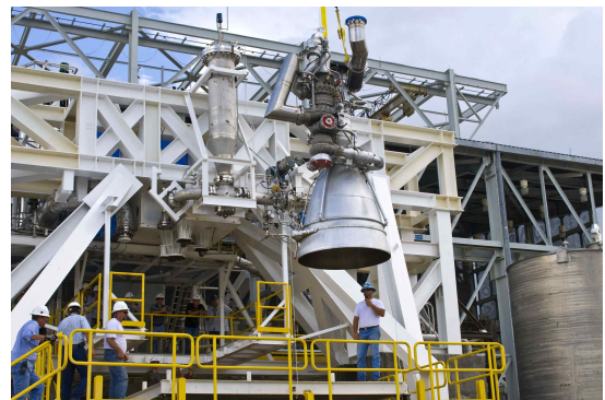
Fig. 1. AJ26-62, 1st stage engine of Antares[3]
