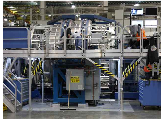
Fig. 3. SpaceX's circumferential Friction Stir Welding(FSW) machine[8]
