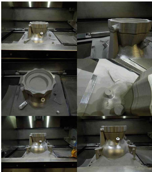
Fig. 9. Super Draco engine in EOS 3D printer[17]
