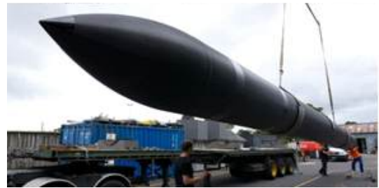
Fig. 23. Carbon composite structures of Electron launch vehicle[50]
